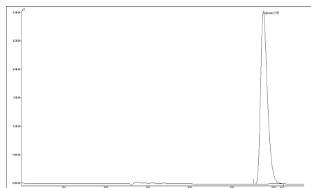
Figure 3: Typical RP- HPLC Chromatogram Brimonidine Tartrate (40 ug /ml) with corresponding retention time.
